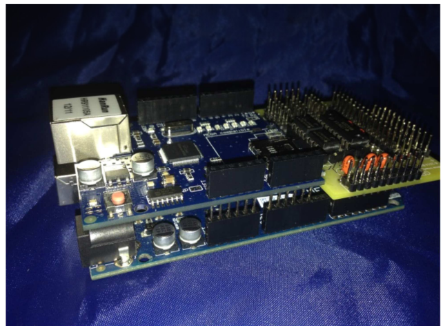
This is the Serial Interface plugged into the Arduino Mega2560+Ethernet
