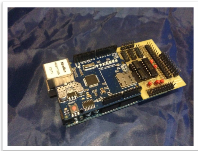
This is the Serial Interface plugged into the Ethermega
